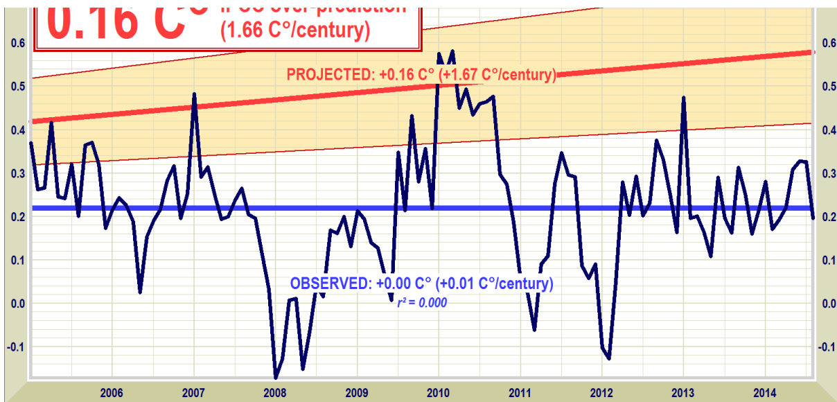
Figure 4. Predicted temperature change, January 2005 to August 2014, at a rate equivalent to 1.7 [1.0, 2.3] C°/century (orange zone with thick red best-estimate trend line), compared with the observed anomalies (dark blue) and zero real-world trend (bright blue), taken as the average of the RSS and UAH satellite lower-troposphere temperature anomalies.
